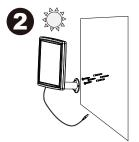
Mark the hole locations of the base of the solar panel (Part B), then set the solar panel (Part B) aside. Check that the marked areas are clear of obstacles such as cables and electrical lines. Drill holes for the enclosed screws and wall anchors. Insert the wall anchors then secure the solar panel in place with the screws.
