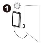
Ensure your solar panel (Part B) is placed so that it can receive direct sunlight for optimal performance. Be aware of objects such as trees or property overhangs that may impede the panel's ability to generate a charge. Adjust the solar panel (Part B) to receive direct sunlight. The solar panel (Part B) is equipped with a 9.84 ft (3m). connecting wire, so the light fixture (Part A) and solar panel (Part B) can be installed up to 9.84 ft (3m) apart.
